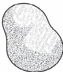
a) nanoparticle (3 ext. dimensions in the nanoscale)
