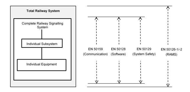
Figure 1 — Scope of the main CENELEC railway application standards
