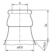
ø between 18,0 mm max. and 16,5 mm min. measured at 3 mm max. down from the top, see key d in Figures 4 and 5. Minimum through Ø bore 15,5 mm.
