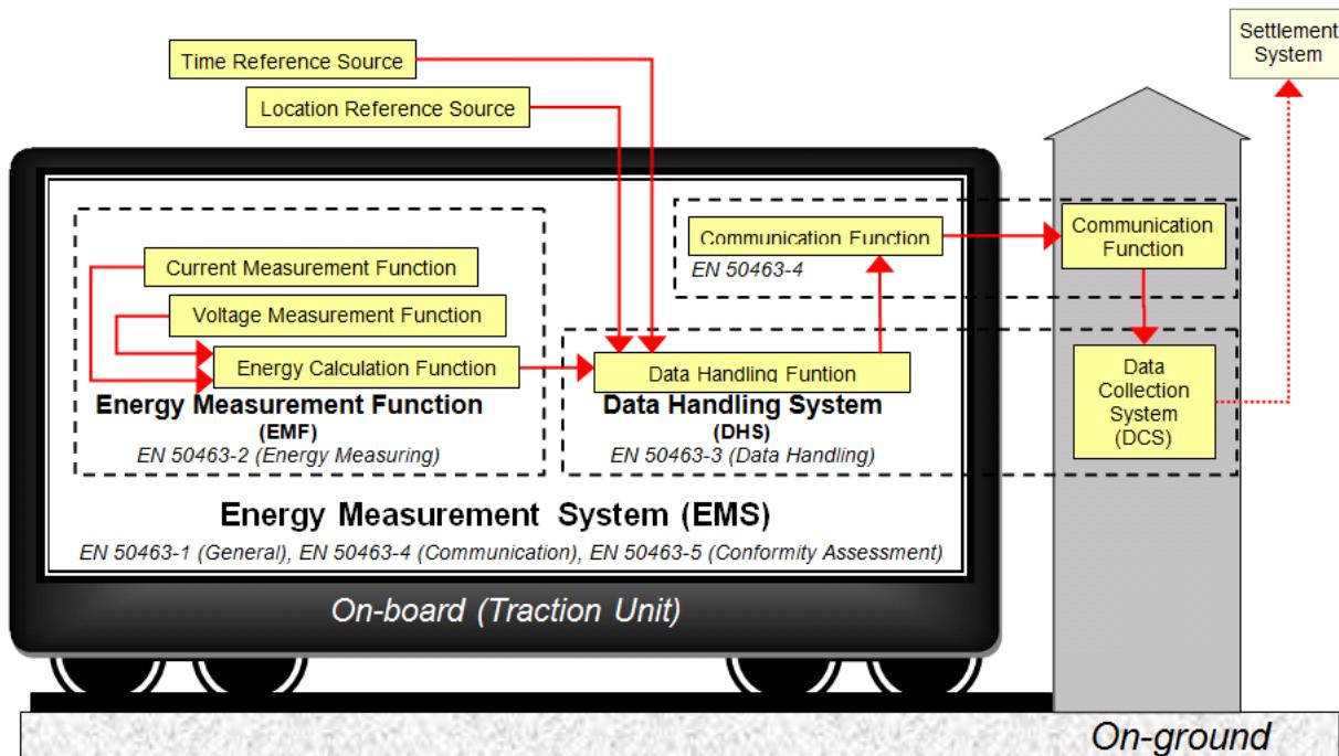
**Figure 1 — EMS functional structure and dataflow diagram**
