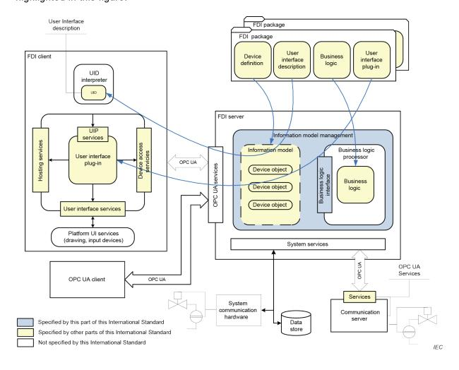
Figure 1 - FDI architecture diagram
