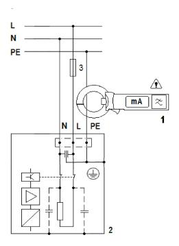
Figure 3e — Example of protective conductor current — direct method with clamp
