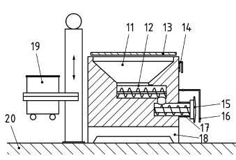
b) Industrial machine with feed intake hopper. protective cover and feeding screw
