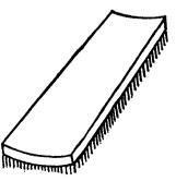
Honeycombing: Separation of the fibres in the interior of timber induced by drying stresses when the outer layers have become casehardened.
