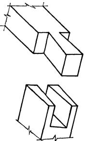
Dowelled joint: A joint in which two members are connected by one or more dowels inserted and glued into counterbalanced drilled holes in the members.
