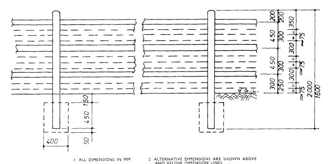
Figure 1. Post and Rail Fence Assembly
