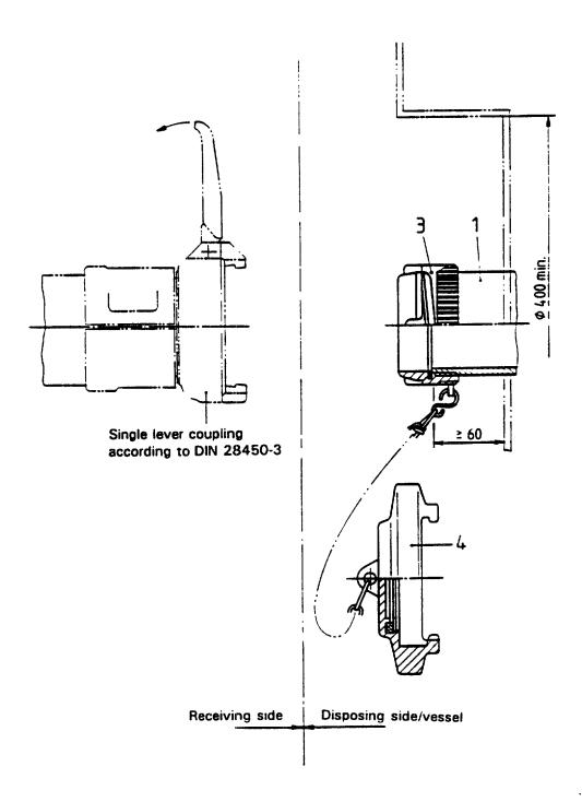
Figure 1: Quick release coupling connection (R)
