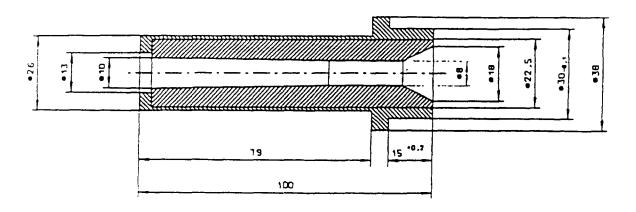
Figure 1: Blasting nozzle
