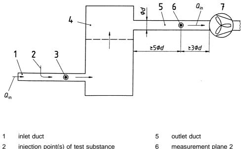
injection point(s) of test substance
