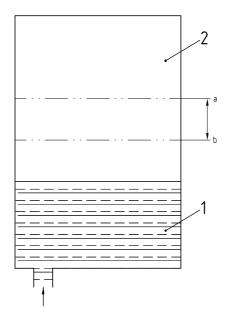
1 oil a p OFF 2 air (gas) b p ON
