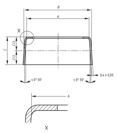
NOTE A is measured at base of radius.
