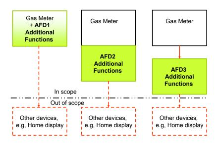
Figure 1 — Additional functionality device
