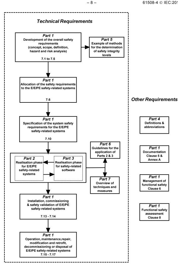
Figure 1 - Overall framework of the IEC 61508 series
