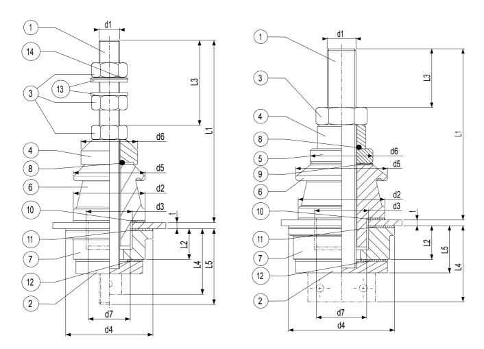
Figure 1 - Type 1 - 3 bushings (250 A to 630 A)
